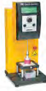
Figure 1: Brookfield CT3 Texture Analyzer for Compression and Tension Testing
