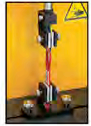
Figure 3: Detail of Package Seal in Dual Grips for Tension Test
