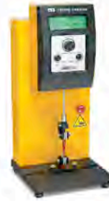
Figure 2: Tension Test on Snack Package Using Brookfield CT3 Texture Analyzer
