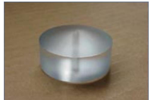
The angled taper of the test probe facilitates product flow and reduces the amount of air-pockets between the probe and sample interface. This helps with the measurement of adhesive characteristics and the movement of particulates between probe perimeter and container.
