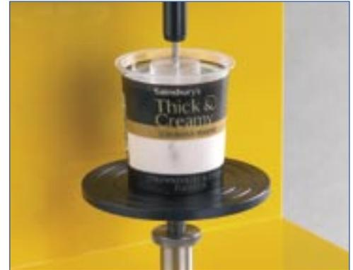
The semi-solid yogurt sample is evaluated in its commercial container. The specially-designed probe is driven into the sample under controlled conditions and a volume of product is displaced. The energy input by the Texture Analyser and the hardness of the sample are key indicators of yogurt quality.
