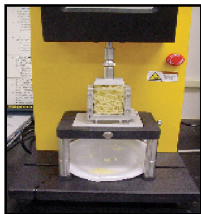
Figure 2: Ramen noodles in Ottawa Cell before Compression Plate begins its Downward Descent
