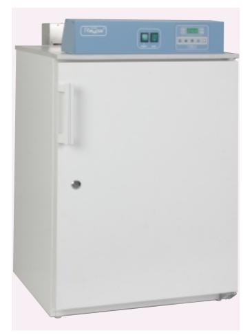
ADJUSTABLE TEMPERATURES FROM 0 °C TO 45 °C. HOMOGENEITY:  $\pm$  1,5°C stability:  $\pm$  0,15°C FORCED AIR CONVECTION.
