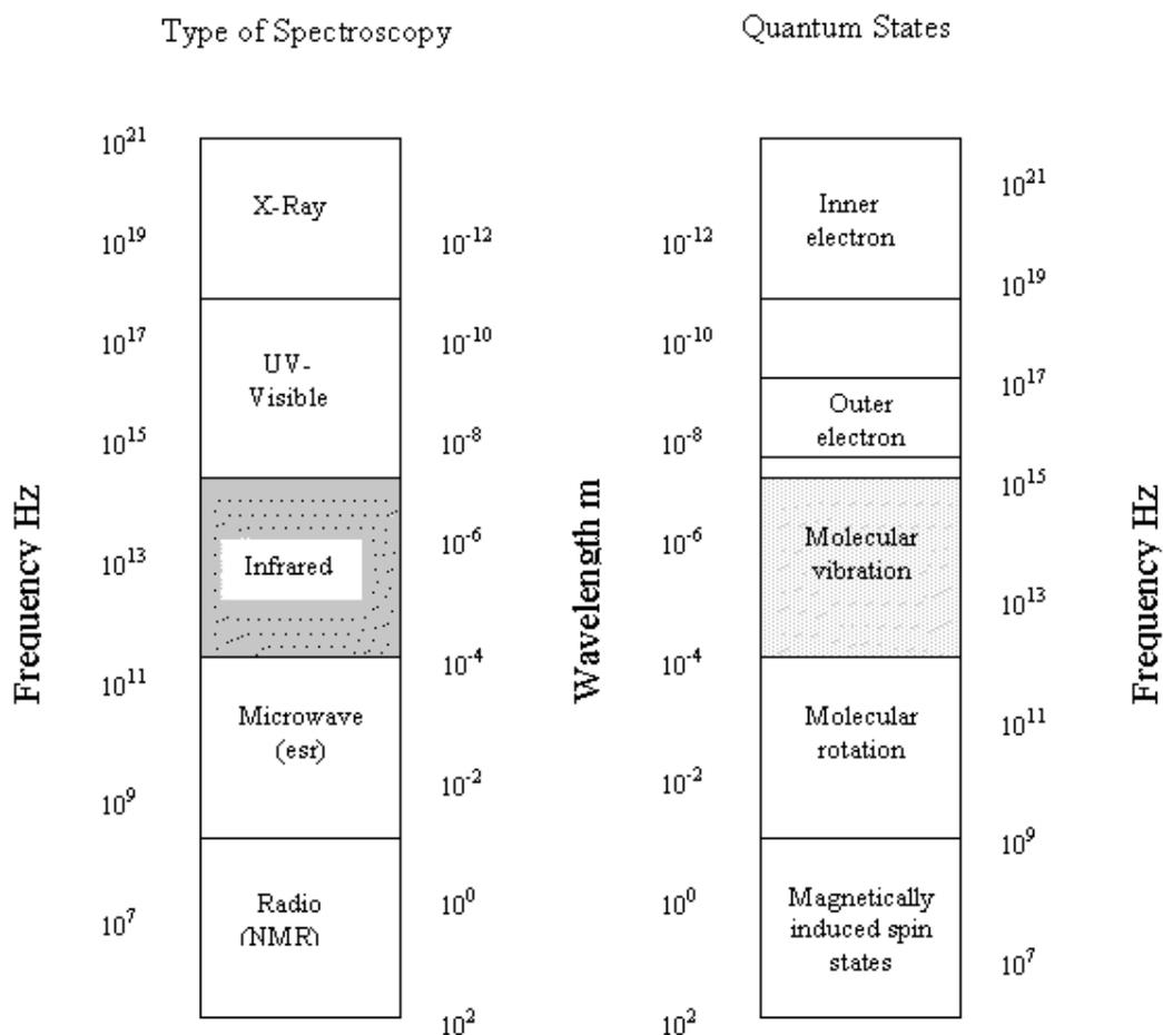
Parts of the electromagnetic spectrum used for spectroscopy.
