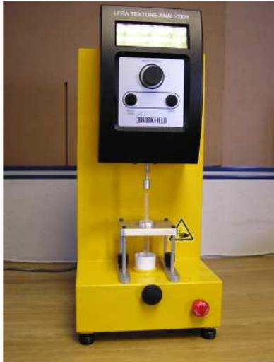
The test rig will quantify the force required to perform extrusion and extraction of an injectable solution using a syringe. The information is important for manufacturers in optimising the quality of the syringe as well as patient comfort and safety.
