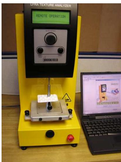
Texture analysis can be used to quantify the force required to extract the tablet from the packaging. Using specialised accessory we are able to imitate a finger pressing on the blister. With the increase in blister packs use for tablet packaging in the pharmaceutical industry it crucial that the packs are easily opened by weak patients and the elderly, but strong enough to avoid accidental opening by children. Texture analysis can be used to quantify the strength of the packaging.
