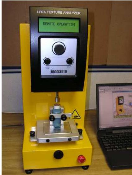
As this involves self-administration its crucial that the inhaler is safe and accurate during drug delivery, Texture analysis to asses the quality and accuracy of the inhaler by using a finger probe to imitate a finger pressing down on the inhaler and measuring the force required to administer a dose.
