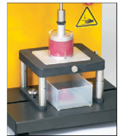
Figure 2: Extrusion Cell for use with CT3 Texture Analyzer
