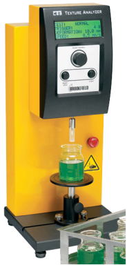
Figure 1: Brookfield CT3 Texture Analyzer
